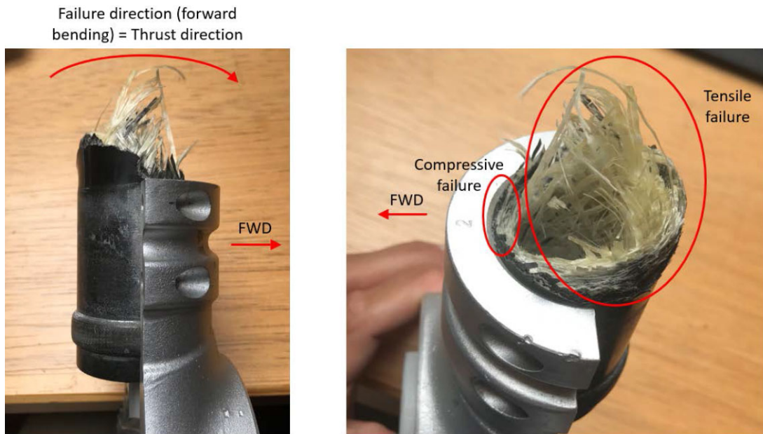
Figure 3 Blade 2 fracture surfaces
