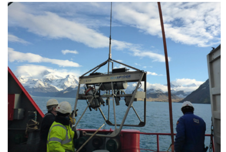
A test deployment of the deep-water camera system from the MV Pharos SG at 300m just outside of Cumberland Bay, South Georgia.
