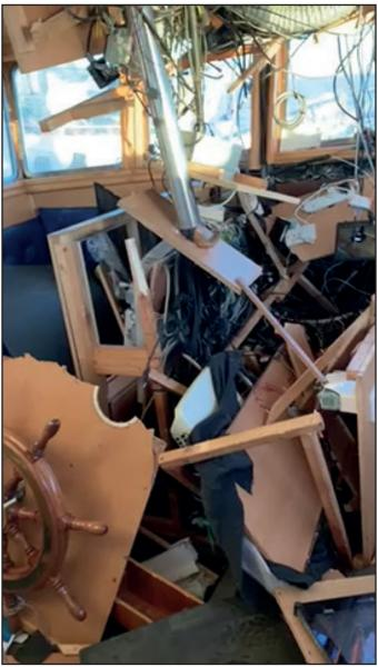
Figure 4: Wheelhouse destruction by shock damage
