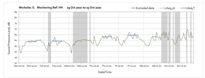
Note: Missing data between 01:00-02:00 on Sunday 25<sup>th</sup> October was due to a technical fault with the monitoring station caused by the clocks going back 1hr at the start of daylight savings.
