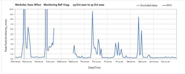
Note: High vibration levels measured throughout the week were due to local disturbance of the vibration monitor and are not representative of HS2 vibration levels. Missing data between 17:00 on Tuesday 21<sup>st</sup> of October and 12:00 on Wednesday 22<sup>nd</sup> of October were due to loss of power at the monitor.
