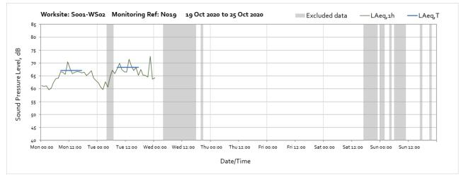
Note: Missing data between 01:00 on Wednesday 21<sup>st</sup> October and 00:00 on Sunday 1<sup>st</sup> November was due to the relocation of the monitor to allow hoarding works to take place. The monitor is awaiting a supply of power at the new location.
