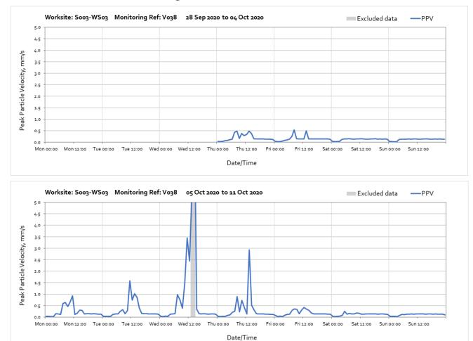
Note: High vibration levels measured at 14:00 on Wednesday 7<sup>th</sup> October were due to local disturbance of the monitor and are not representative of HS2 vibration levels.
