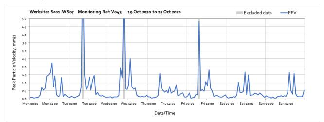
Note: High vibration levels measured between 10:00 and 11:00 on Tuesday 22<sup>nd</sup> of September were due to local disturbance of the monitor and are not representative of HS2 vibration levels.
