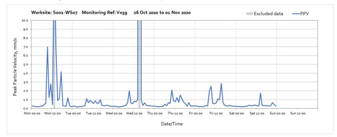
Note: High vibration levels measured throughout the week were due to local disturbance of the vibration monitor and are not representative of HS2 vibration levels.
