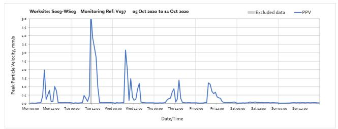
Note: High vibration levels measured at 11:00 on Tuesday 6<sup>th</sup> October were due to local disturbance of the monitor and are not representative of HS2 vibration levels.
