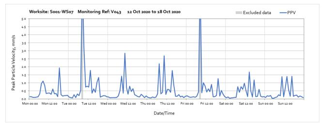
Note: High vibration levels measured throughout the week were due to the use of the neraby residential bin store and are not representative of HS2 vibration levels.
