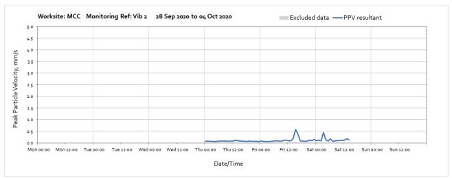
Note: Missing data from 15:00 on 3<sup>rd</sup> October 2020 was due to loss of the signal, the monitor has since been upgraded to a more stable data connection.
