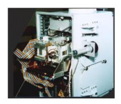
The sieve pack unit should be pulled forward. pack.
