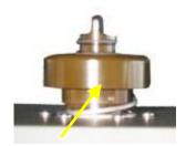
Wipe the inlet port under the rain cap assembly
