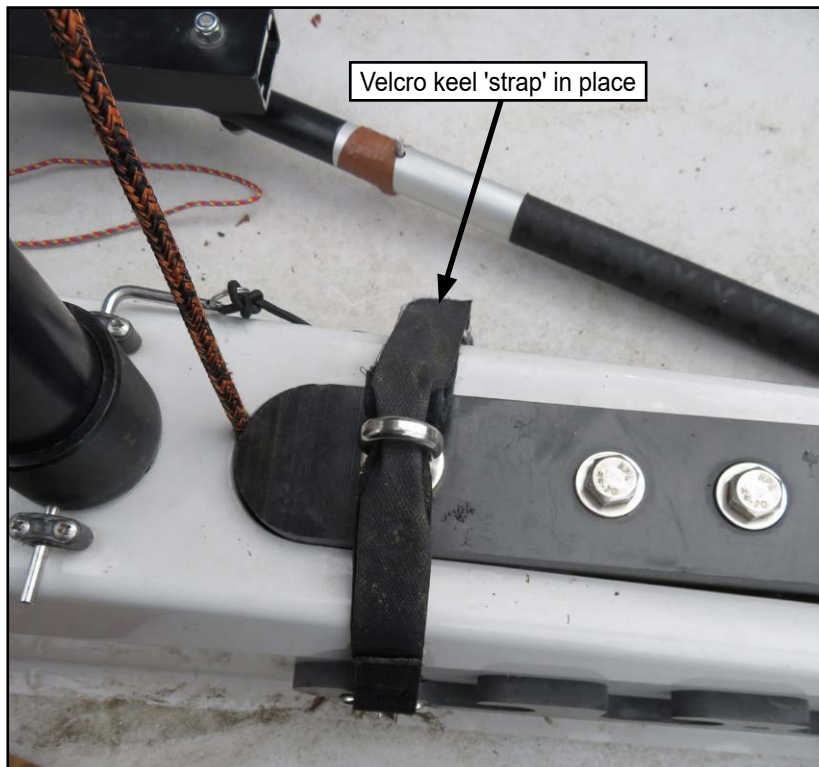
Figure 8: The Velcro™ keel strap
