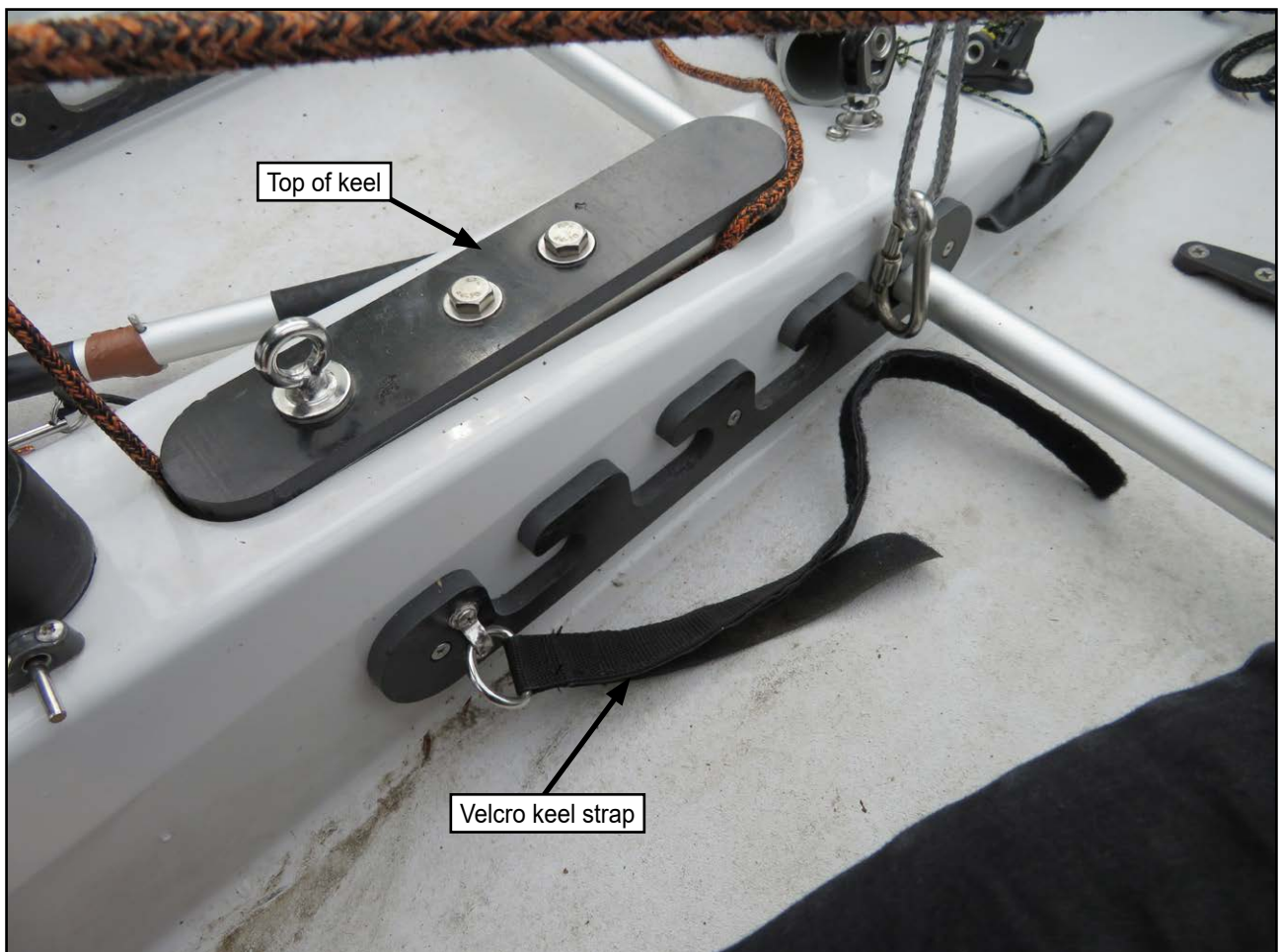
Figure 9: RSVC 307's keel strap as found after the accident (note: jib sheet caught in keel housing as the boat was righted)
