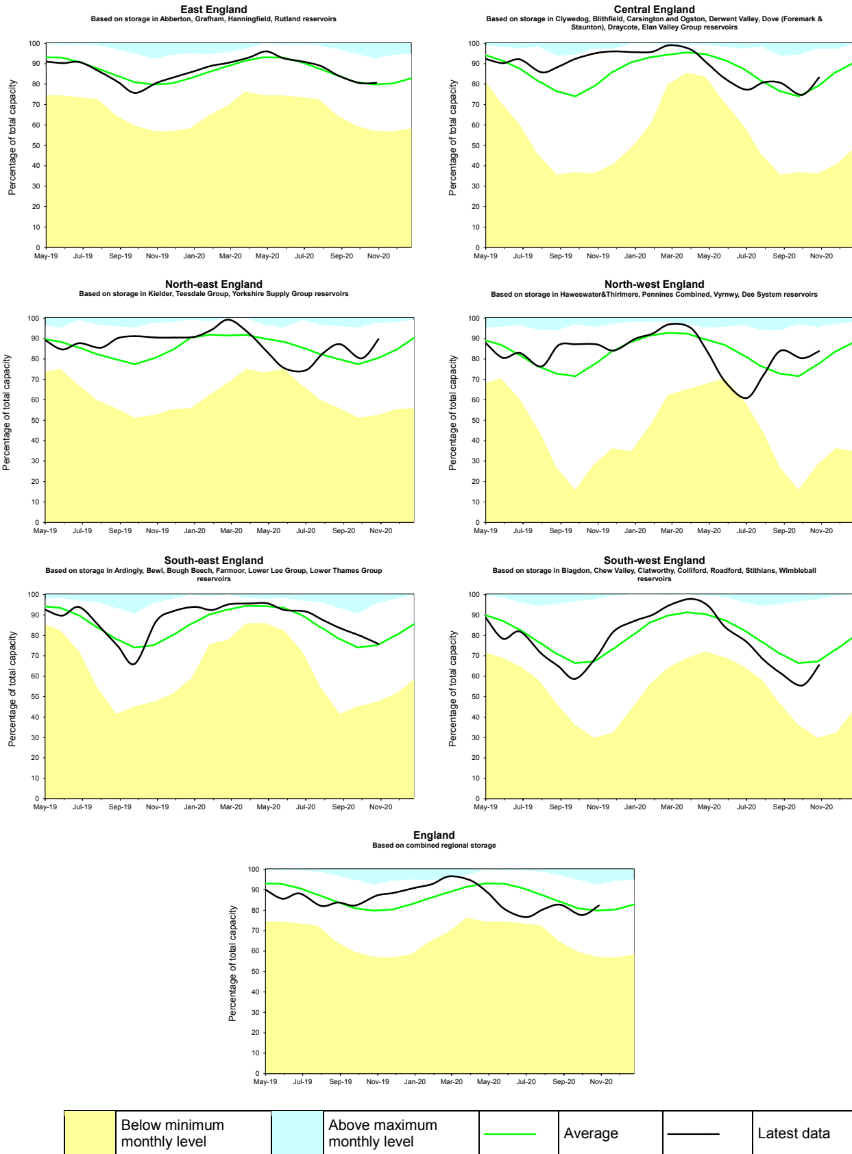
Figure 5.2: Regional reservoir stocks. End of month reservoir stocks compared to long term maximum, minimum and average stocks (Source: Water Companies). Note: Historic records of individual reservoirs/reservoir groups making up the regional values vary in length.
