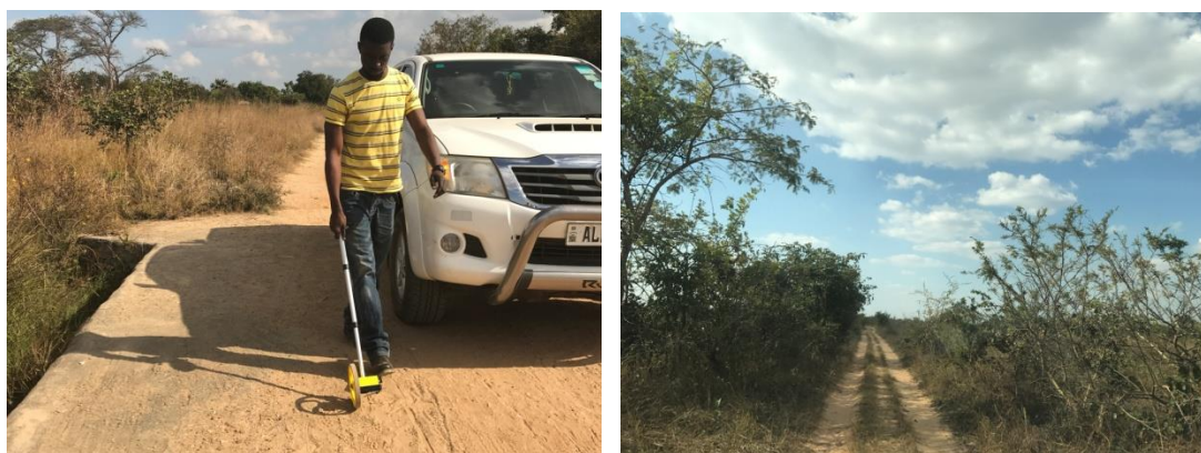
FIGURE 6.2 - SURVEY TEAMS CARRYING OUT ROAD CONDITION SURVEY IN CHONGWE DISTRICT
