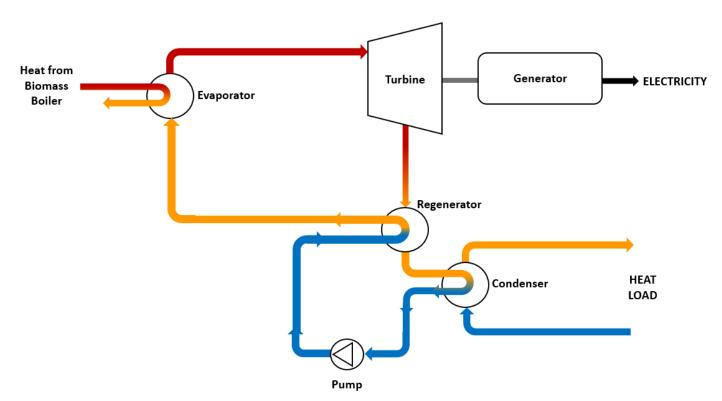
Figure 1: Organic Rankine Cycle (ORC) working principle
