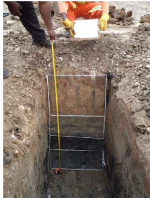
Figure 4-7: Logging of subgrade profile
