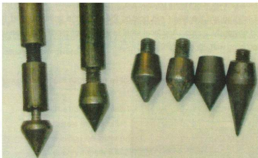
Figure 4-9: Typical cones and problems
