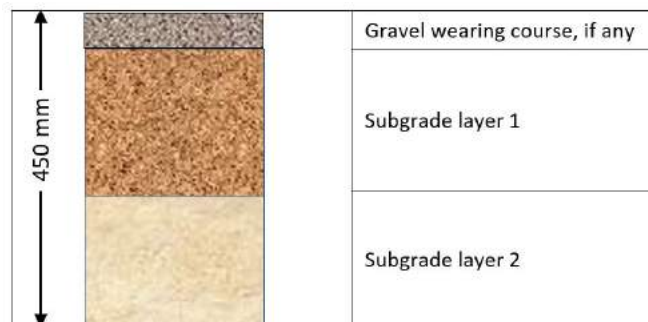
Figure 4-6: Typical soil profile in test pit
