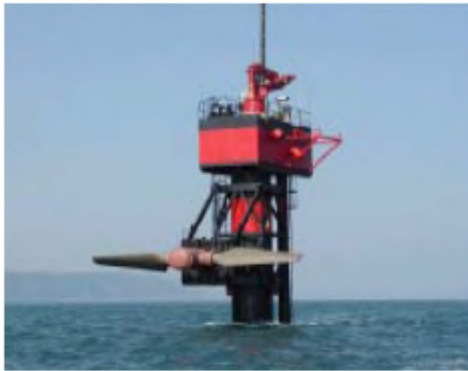
“Seaflow” project – tidal turbine installation. Coloured red and black as isolated danger. (Photos courtesy Marine Current Turbines Ltd.)
