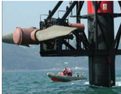
“Seaflow” project – tidal turbine installation. Coloured red and black as isolated danger. (Photos courtesy Marine Current Turbines Ltd.)
