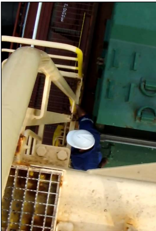
Figure 15: Reconstruction showing size of the gap between the ladder platform and the stacked hatch covers
