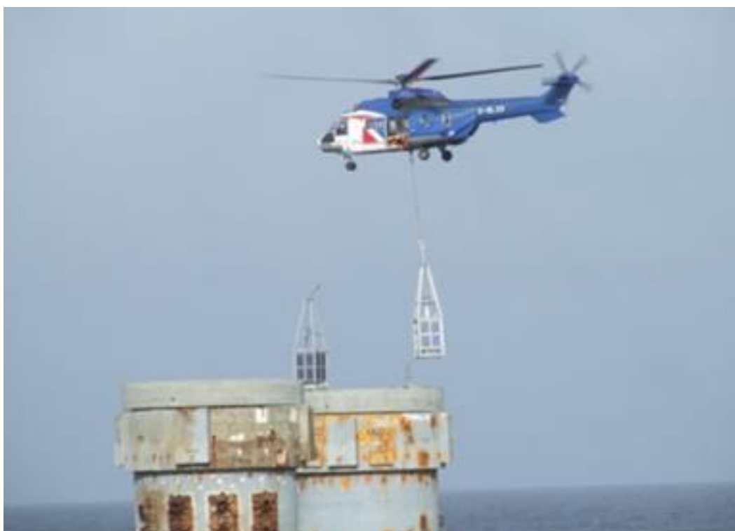
Figure 2-3 AtoN deployment via helicopter
