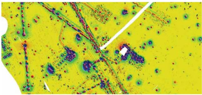
Magnetic results showing former structures and possible areas of concern on the former MOD site © Crown
