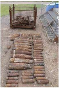
Items of ordnance recovered as a result of towed array surveys on a former firing range © Crown
