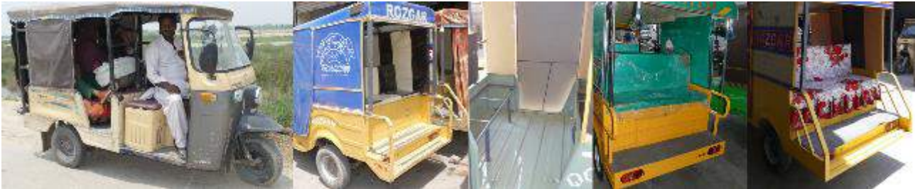
Figure 13 Examples of 6-seater and 9-seater auto-rickshaws with 'Qingqi'-type rear-facing seats
