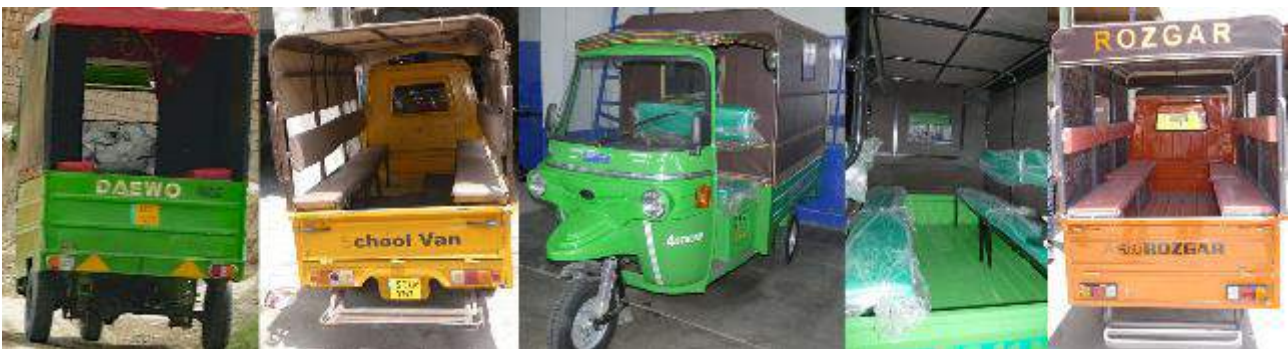
Figure 14 Examples of auto-rickshaws with sideways-facing seats often used to carry school children
