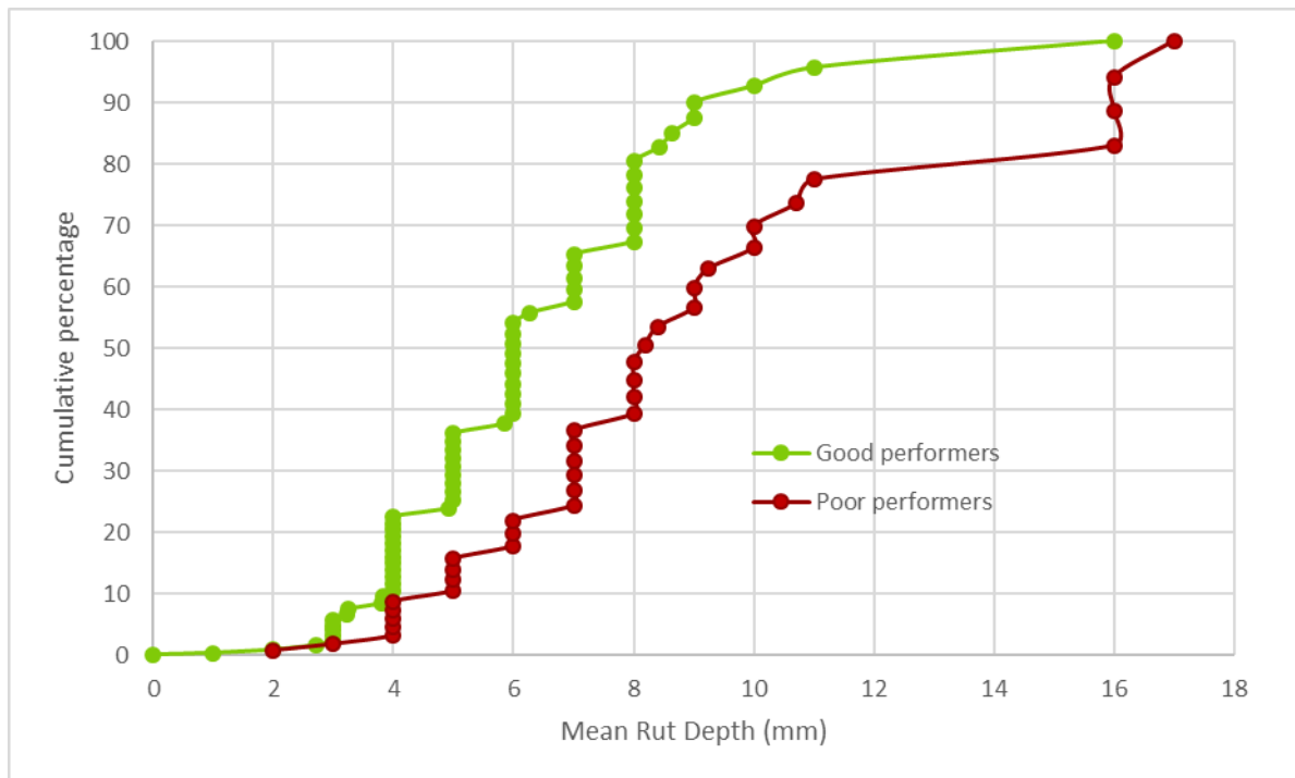
Figure 1 Cumulative frequency distributions of mean rut depths of sections used in the analysis
