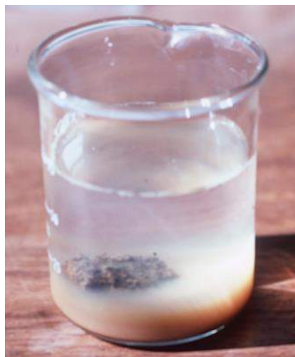
Figure B.4 Dispersive soil in water (crumb test) showing suspension that does not settle out
