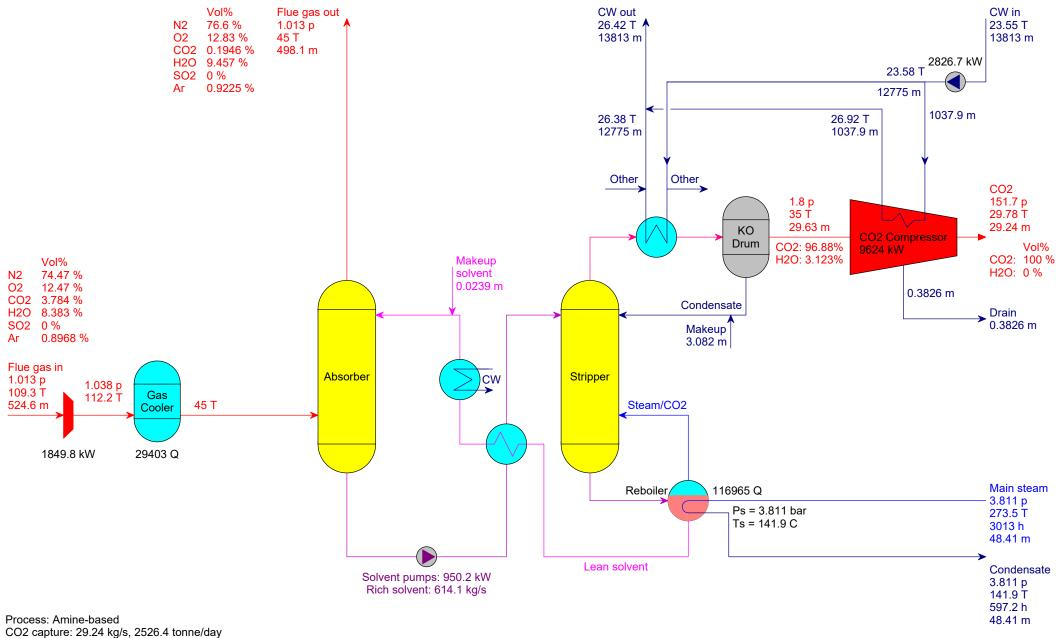
Process: Amine-based CO2 capture: 29.24 kg/s, 2526.4 tonne/day CO2 capture efficiency: 95 % Heat input: 116965 kW, 117 MW, 4000 kJ/kg CO2 Total electrical power consumption: 15541 kW Solvent consumption: 2.069 tonne/day
