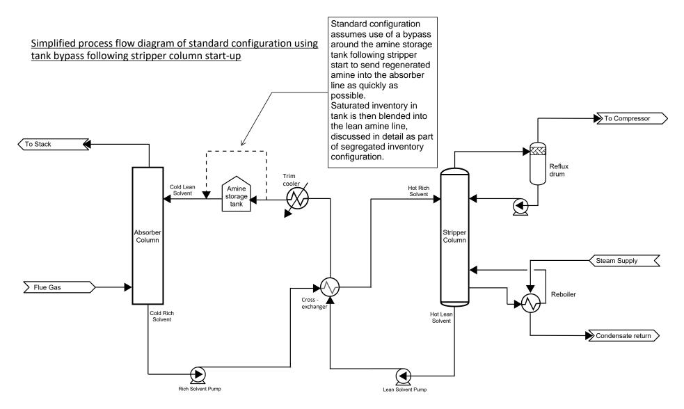
Figure 3. Standard configuration followed by tank bypass when stripper column start-up is complete
