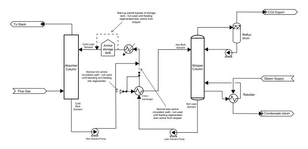
Simplified process flow diagram of improved configuration after start-up
