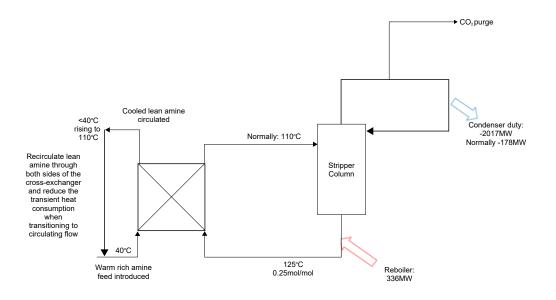
Figure 11. Introducing feed of new rich amine to cross-exchanger and extracting hot lean amine
