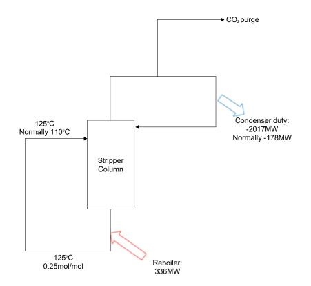
Figure 8. Recycling of stripper inventory leading to rising condenser duty
