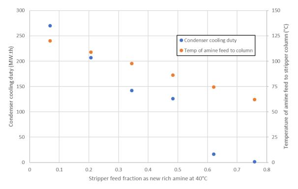
Figure 12. Effect on feed temperature and condenser duty by blending various fractions of rich amine at 40°C into stripper feed
