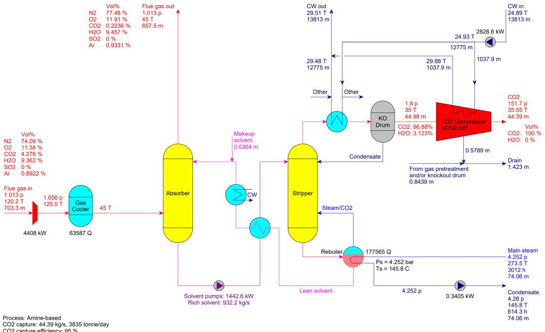
CO2 capture: 44.39 kg/s, 3835 tonne/day CO2 capture efficiency: 95 % Heat input: 177565 kW, 177.6 MW, 4000 kJ/kg CO2 Total electrical power consumption: 23827 kW Solvent consumption: 3.144 tonne/day
