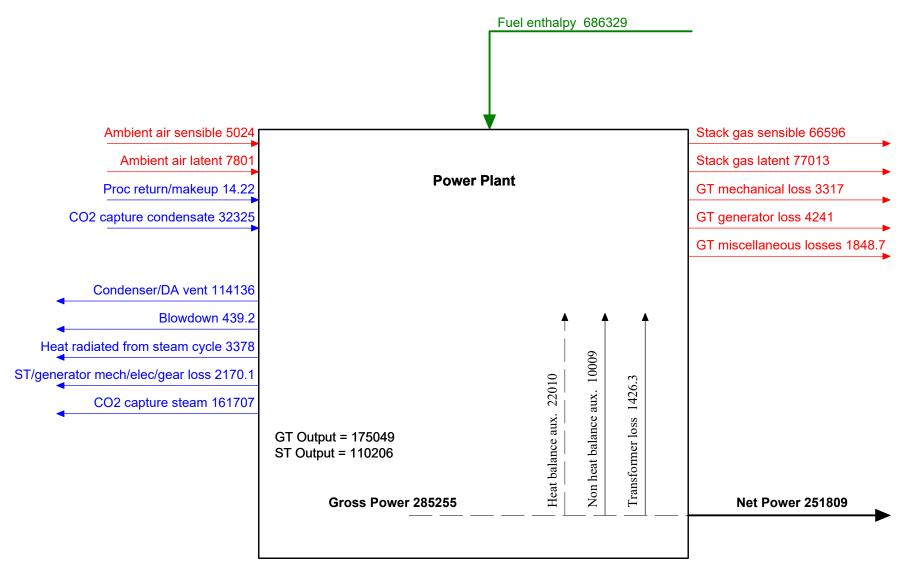
Zero enthalpy: dry gases & liquid water @ 32 F (273.15 K)
