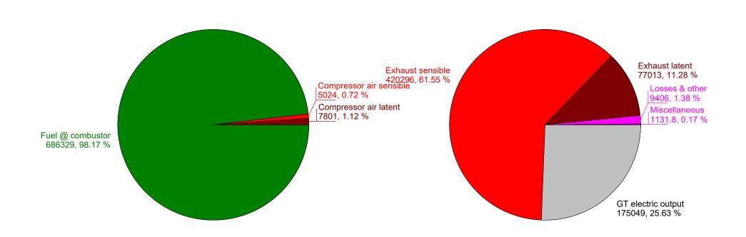
Zero enthalpy: dry gases & liquid water @ 32 F (273.15 K)
