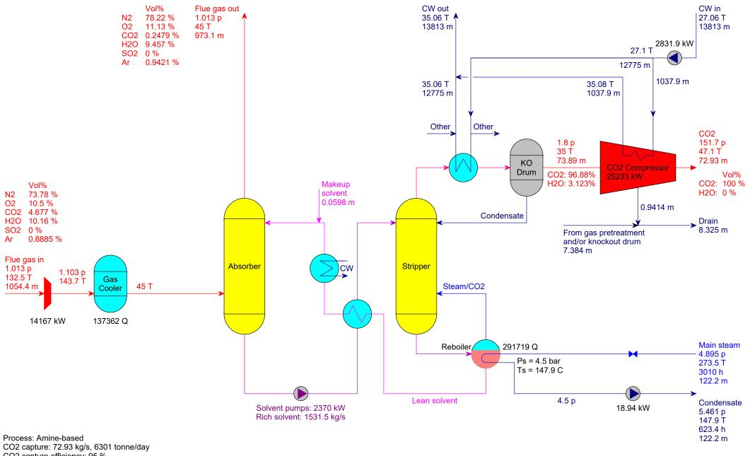
CO2 capture: 72.93 kg/s, 6301 tonne/day CO2 capture efficiency: 95 % Heat input: 291719 kW, 291.7 MW, 4000 kJ/kg CO2 Total electrical power consumption: 45345 kW Solvent consumption: 5.168 tonne/day
