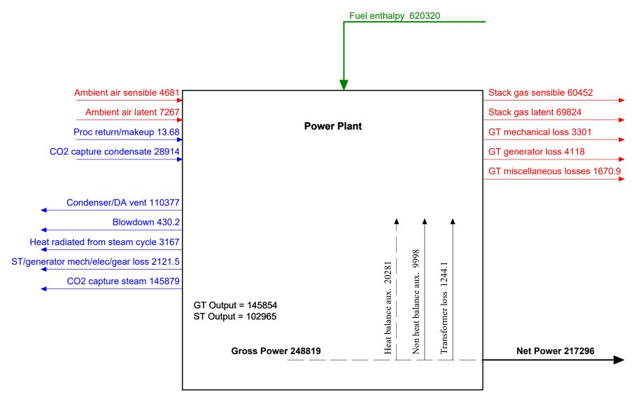
Zero enthalpy: dry gases & liquid water @ 32 F (273.15 K)
