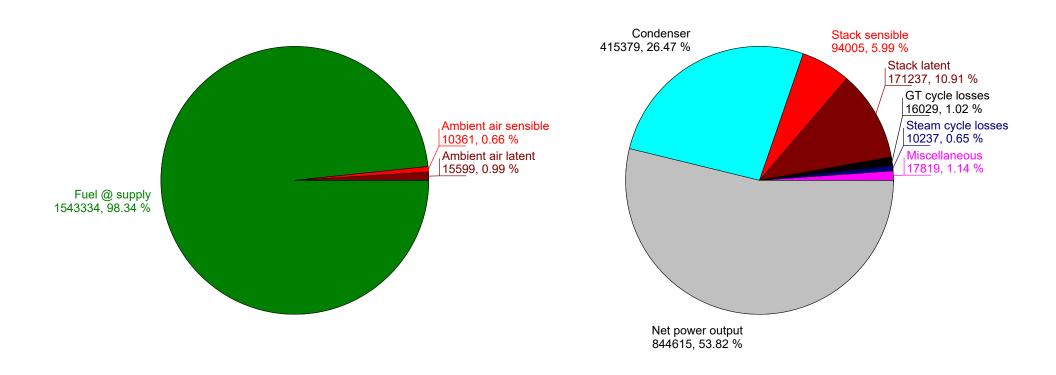
Zero enthalpy: dry gases & liquid water @ 32 F (273.15 K)
