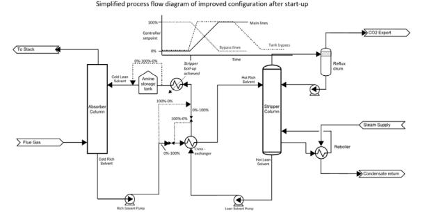
Figure 7. Segregated amine inventory configuration: transitioning from bypass flows to circulating flow once stripper boil-up is achieved
