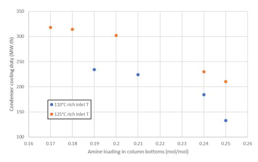
Figure 9. Increasing condenser duty as stripper amine loading drops from initial 0.25 mol/mol
