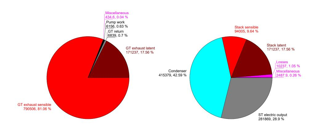
Zero enthalpy: dry gases & liquid water @ 32 F (273.15 K)
