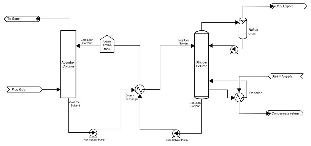
Figure 2. Post-combustion capture process considered for 'standard configuration'
