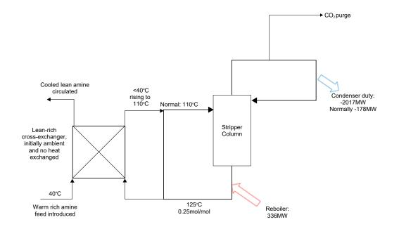
Figure 10. Introducing feed of new rich amine to cross-exchanger and extracting hot lean amine
