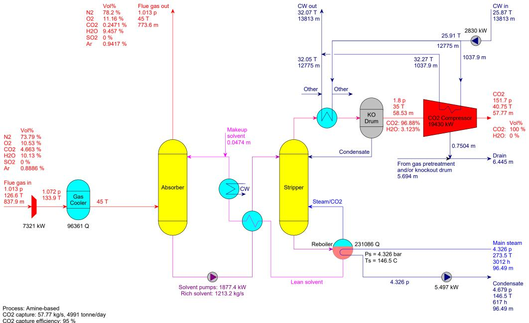
CO2 capture: 57.77 kg/s, 4991 tonne/day CO2 capture efficiency: 95 % Heat input: 231086 kW, 231.1 MW, 4000 kJ/kg CO2 Total electrical power consumption: 32037 kW Solvent consumption: 4.093 tonne/day
