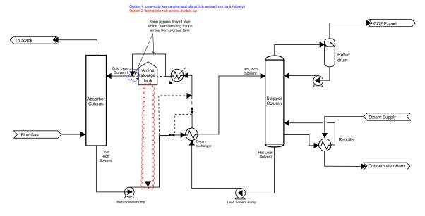
Figure 17. Using a single tank with varying bypass rates in combination with segregated solvent inventory
