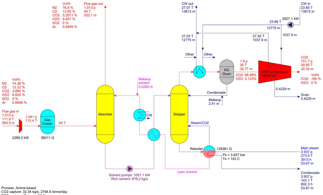
CO2 capture: 32.34 kg/s, 2794.6 tonne/day CO2 capture efficiency: 95 % Heat input: 129381 kW, 129.4 MW, 4000 kJ/kg CO2 Total electrical power consumption: 17139 kW Solvent consumption: 2.289 tonne/day
