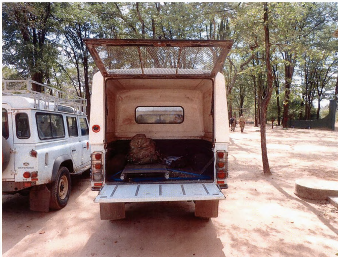
Figure 1.4. 16. Land Rover 130 rear cab equipped with stretcher and medical Bergen
