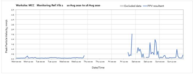
Note: Missing data between 21:00 on 12<sup>th</sup> August 2020 and 15:00 on 14<sup>th</sup> August 2020, 21:00 on 14<sup>th</sup> August 2020 and 00:00 on 15<sup>th</sup> August and 15<sup>th</sup> August 09:00 were due to loss of power caused by abnormal battery consumption.
