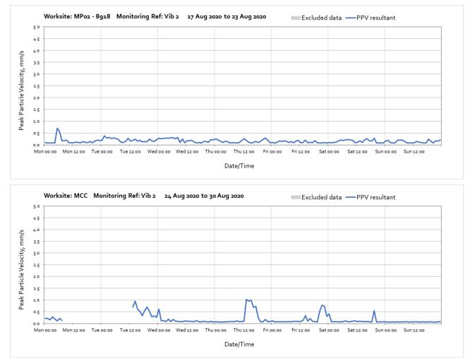
Note: Missing data between 08:00 on 24<sup>th</sup> August 2020 and 12:00 on 25<sup>th</sup> August 2020 was due to loss of power caused by abnormal battery consumption.
