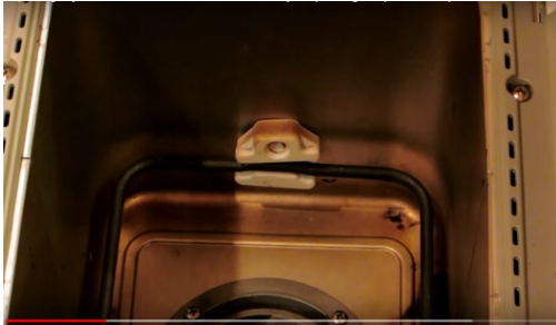
Figure 11: Damaged Ceramic Bobbin in Unit
