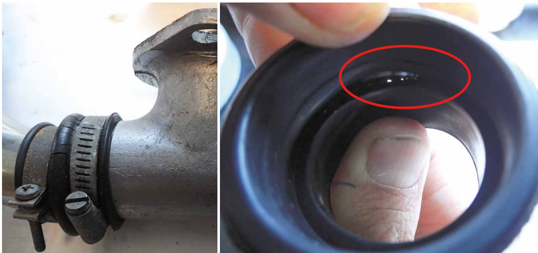
Figure 7 Inlet manifold flexible joint
