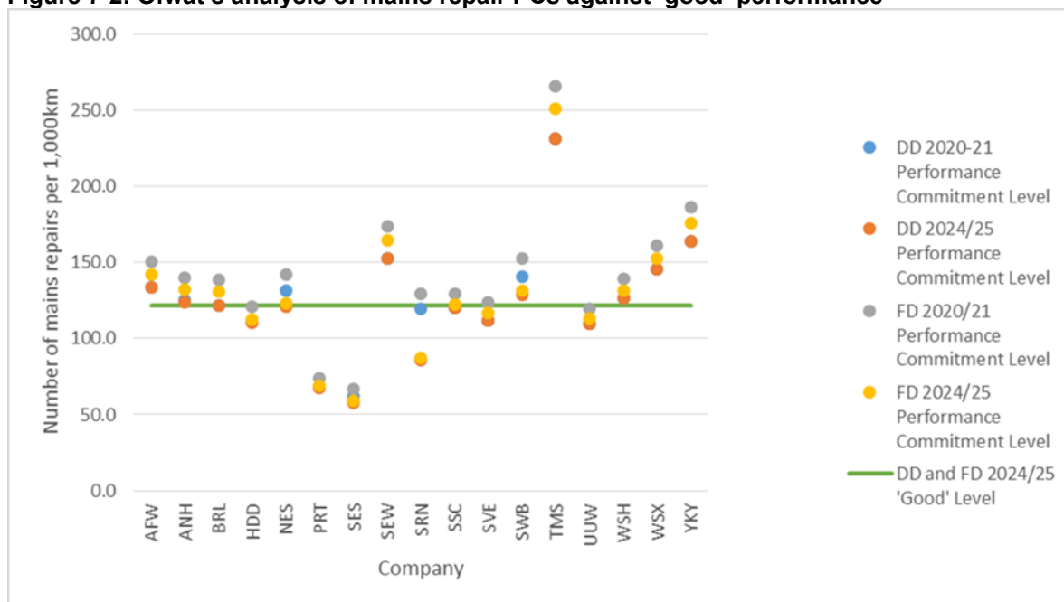
Figure 7-2: Ofwat's analysis of mains repair PCs against 'good' performance
