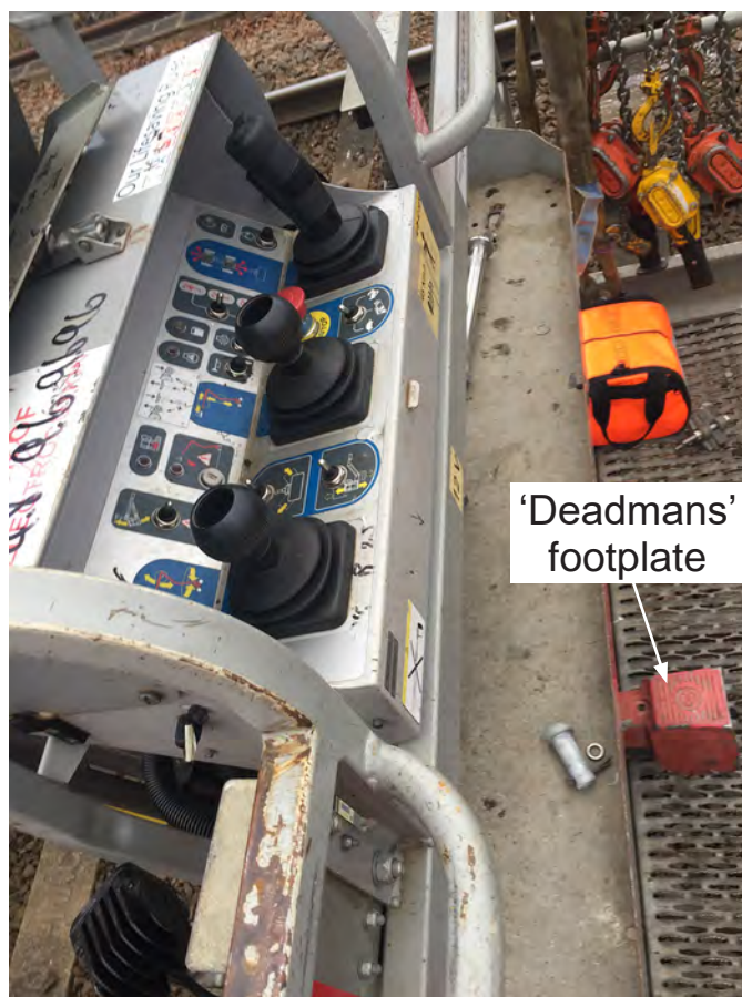
Figure 8: The control console and 'deadmans' foot control on MEWP 10
