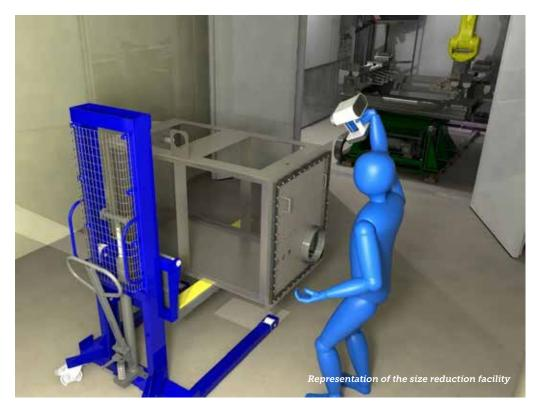
Gloveboxes used for research, development and operations that have come to the end of their life will be decommissioned as part of the site's clean-up programme. Many of these are contaminated with alpha bearing material and current decommissioning plans include manual techniques which are often hazardous and time consuming. There is a driver to address this challenge using alternative technologies to deliver safer, more efficient decommissioning at a lower cost.
