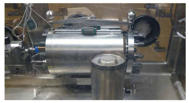
The image above shows the can puncture and gas sampling rig with an unpunctured outer can in the foreground. In support of the underpinning science to understand how packages will evolve over time, this equipment is used for puncturing SNM packages so that gases in the head space of the outer can may be analysed (Courtesy of the National Nuclear Laboratory).
