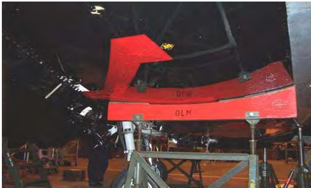
Figure 26 – Example OLM specific ground equipment ('OLM' wing trestles over strain gauges)
