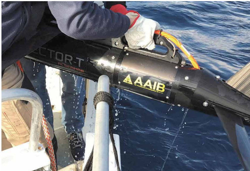
The towed fish being recovered from the water during sea trials
