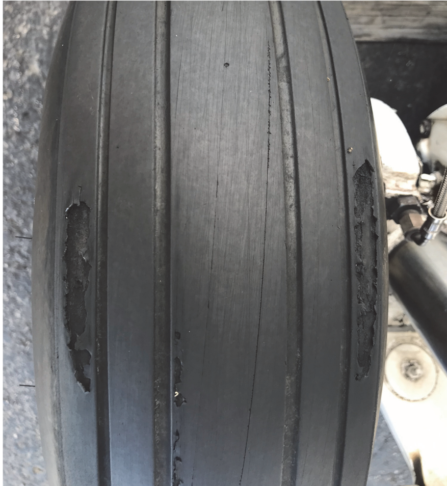
Figure 4 Tyre wear and damage
