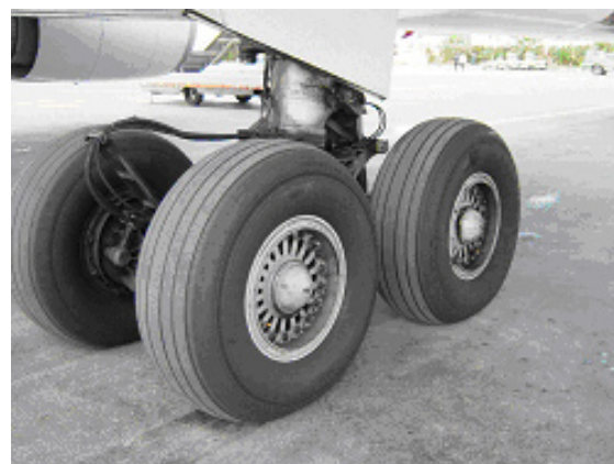
Commercial aircraft tyres can be pressurised to 250 psi, and can deflate explosively if damaged by fire and/or impact
