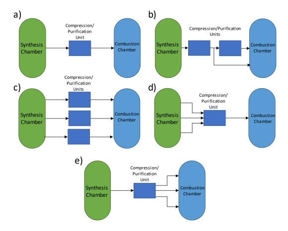
Figure 2. Examples of <u>non-compliant</u> configurations. The lines in red show paths where the *Advanced Fuel* does not pass through the *Compression Unit(s)* or *Purification Unit(s)* when being transported from the *Synthesis Chamber* to the *Combustion Chamber*
