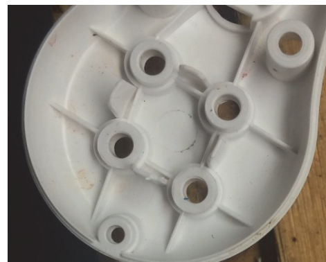
Undamaged motor mount
