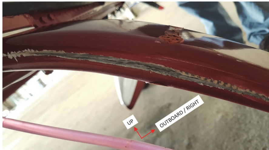
Figure 1 Damage to right MLG leg
