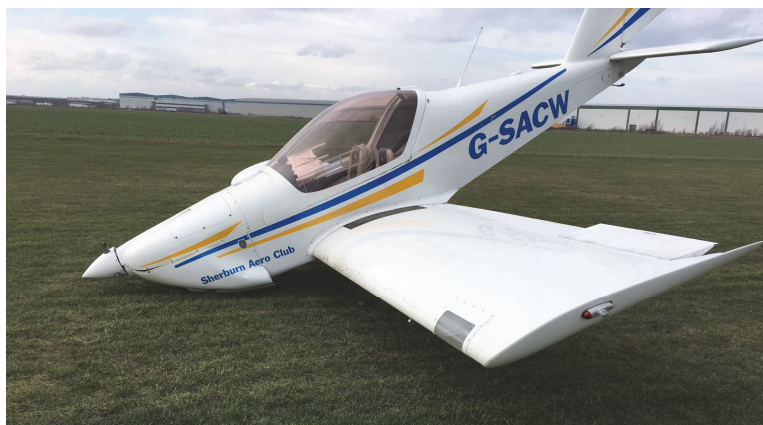
Figure 1 G-SACW nosewheel detached
