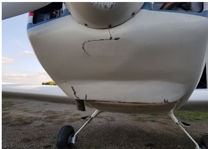
Figure 1 Damage to nose fairing and spinner
