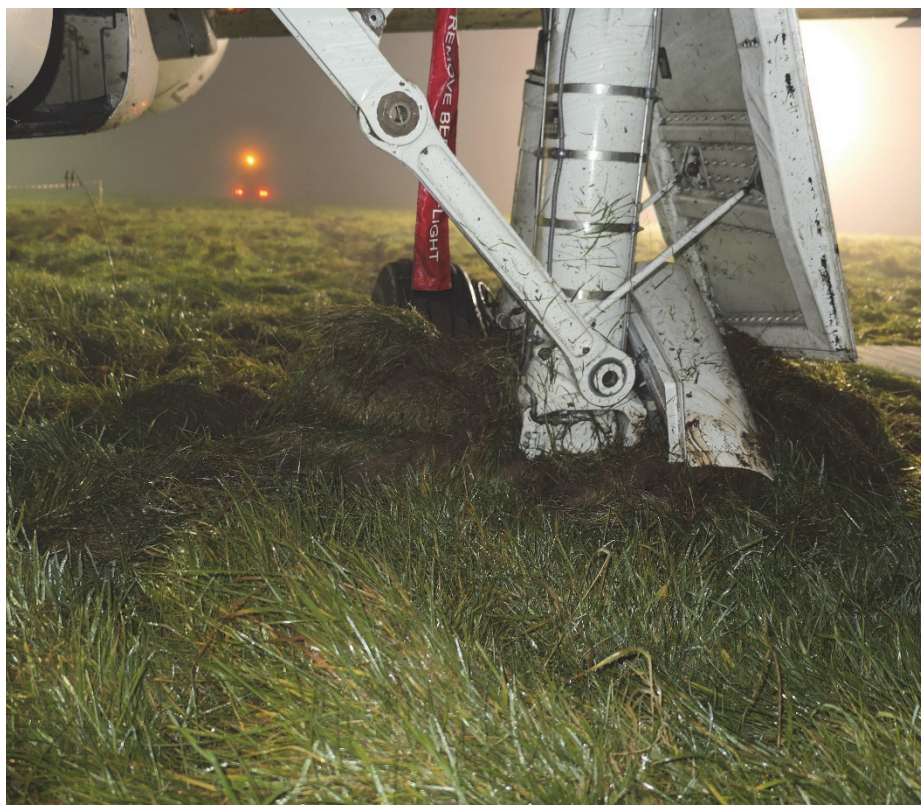
Figure 6 The extent of the entrapment of the main wheels and landing gear (left side shown, the right side was similar)
