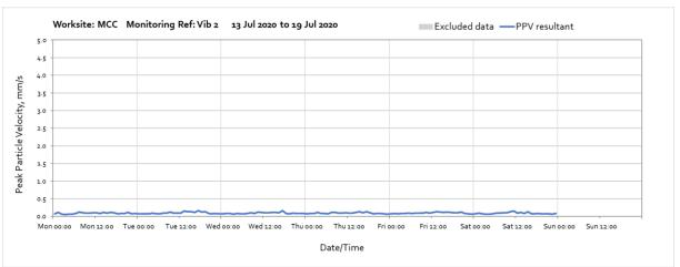
Note: Missing data between 00:00 on Sunday 19<sup>th</sup> July until the end of the month was due to the removal of the monitor from site for routine maintenance (calibration).
