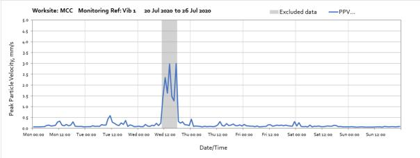
Note: High vibration levels measured between 11:00 and 17:00 on Wednesday 22<sup>nd</sup> July were due to local disturbance of the monitor.
