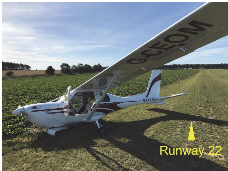
Figure 1 G-CEOM gear collapse
