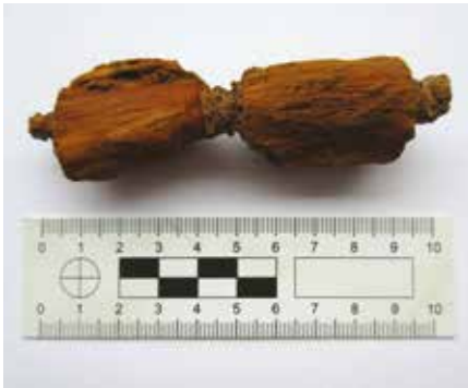
A set of wooden rollers from an early spinning machine © Holcombe Moor Heritage Group
