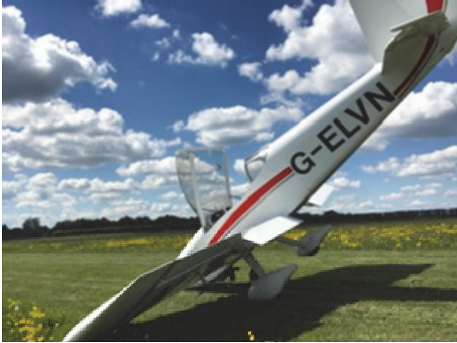
Figure 1 G-ELVN nose gear collapsed
