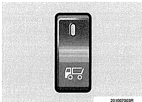
Fig 12 Tail lift platform switch
