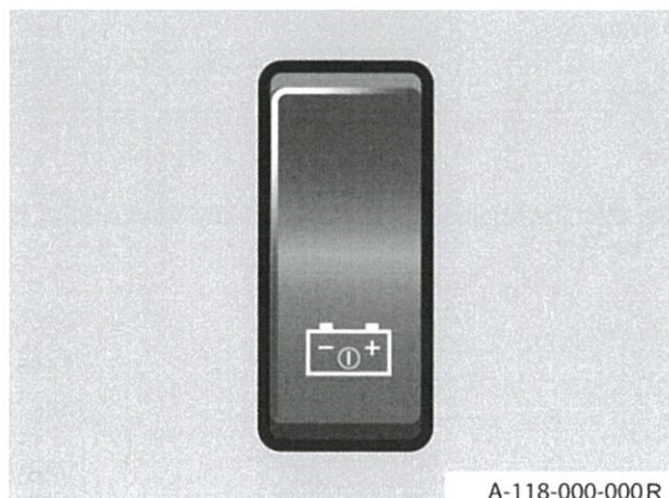
Fig 2 Electrical battery master switch
