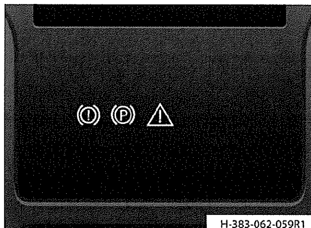
Fig 11 Parking brake malfunction
