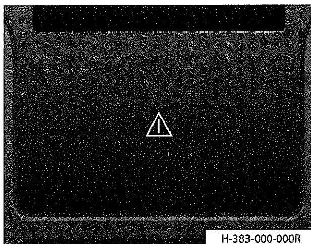
Fig 34 Central warning light
