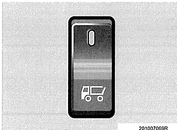
Fig 1 Tail lift platform switch
