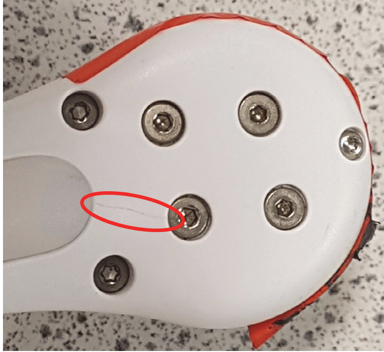
Figure 4 Example of motor attachment cracking
