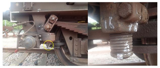
Figure 18: Typical split nut and eyebolt condition on wagon MPA 394228
