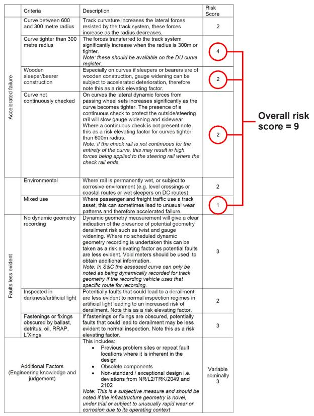
Figure 10: Example consideration of Network Rail's derailment risk assessment criteria for the Up High Level line at 0 miles 27 chains. Table taken from procedure: 'How to determine higher or unusual risk of derailment on track assets'.
