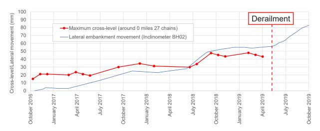
Figure 17: Development of the maximum cross-level around 0 miles 27 chains compared to the lateral embankment movement measured at ground level at inclinometer BH02
