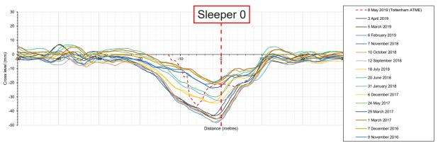
Figure 11: Track geometry measurements showing the gradual formation of the cross-level feature close to 0 miles 27 chains on the up High Level line and how this compared with the feature that the Tottenham ATME measured after the derailment.
