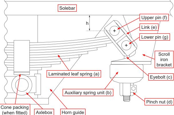
Figure 9: Suspension unit arrangement
