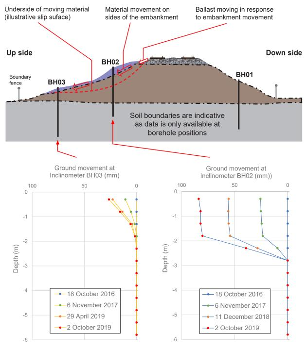
Figure 14: Cross-section of Mitre Bridge Curve embankment showing illustrative slip surface and simplified ground movement. Graphs show how the lateral movement measured at inclinometers BH02 and BH03 varied with borehole depth.
