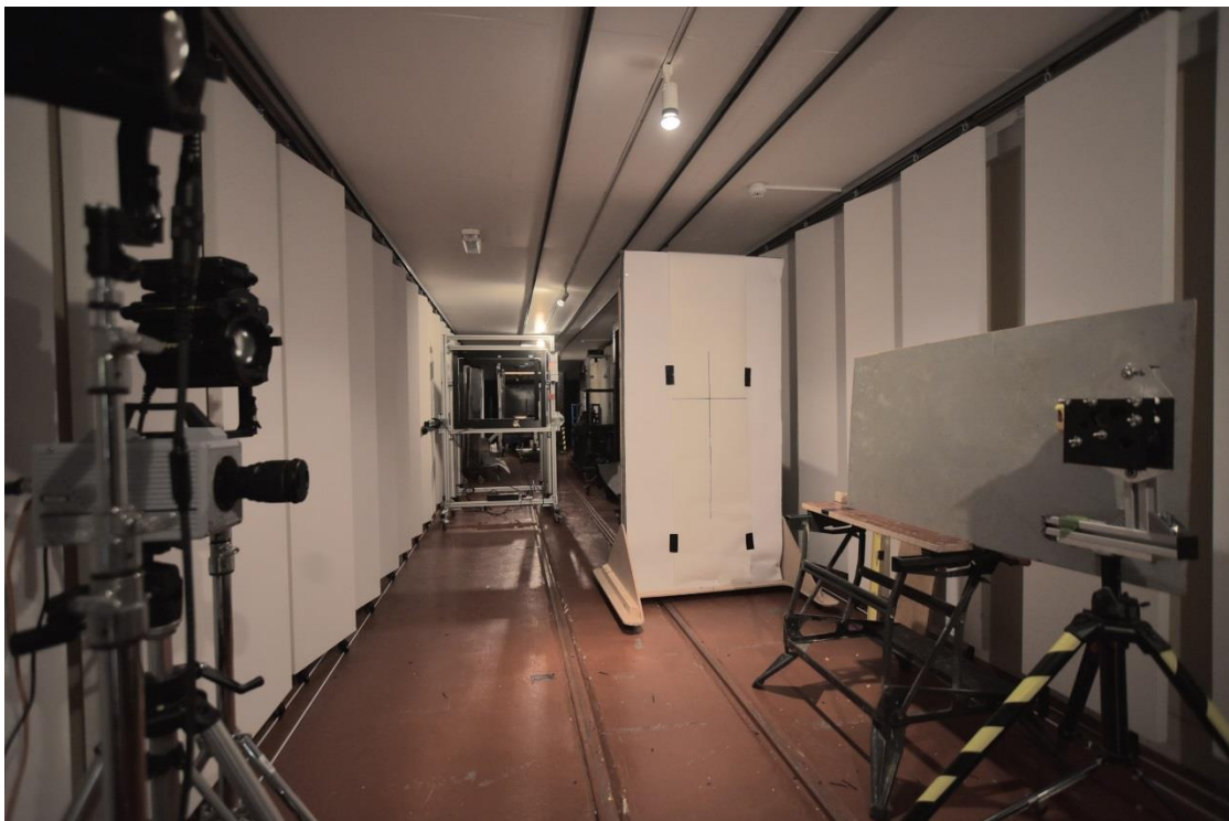
Figure 64: TASER 7™ probe velocity measurement trial set-up
