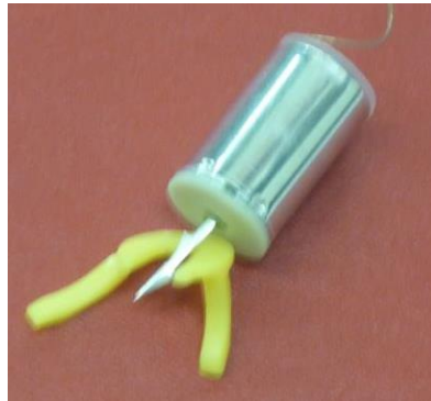
Figure 72: TASER 7™ operational probe with trapped ejector
