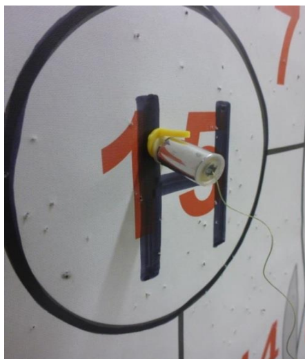
Figure 73: TASER 7™ operational probe embedded in target with a trapped ejector
