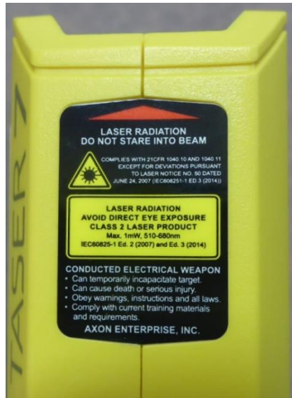
Figure 70: Laser warning label on TASER 7™
