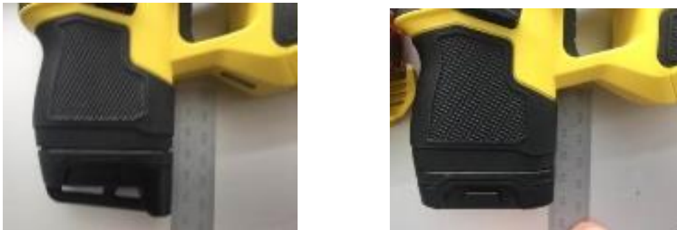
Figure 3: TASER 7™ battery options (tactical on the left and compact on the right)
