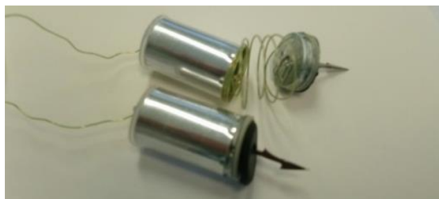
Figure 8: Operational probe showing the wire spooled inside the probe body and the break-away probe design (top)
