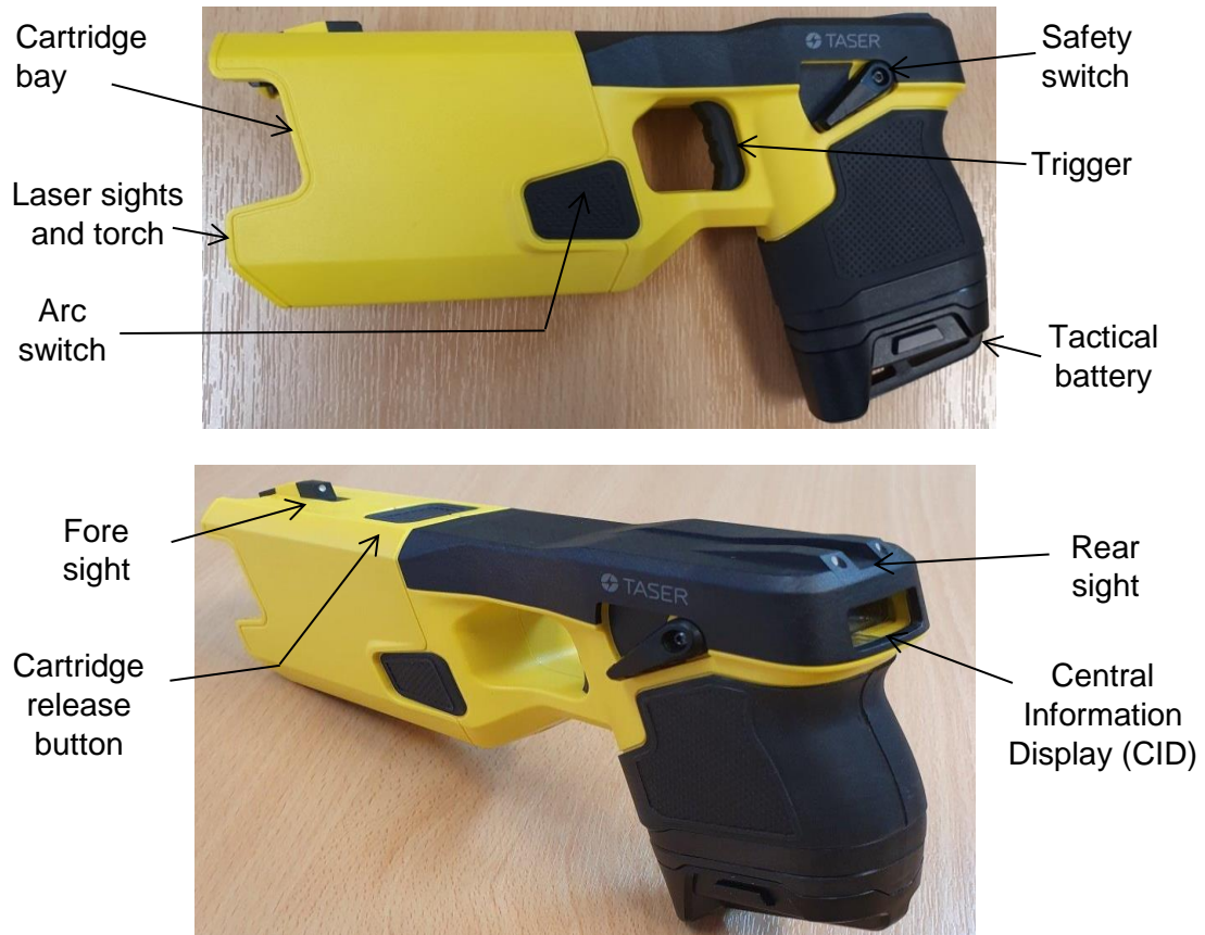
Figure 1: TASER 7™ handle with tactical battery inserted
