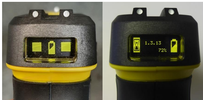
Figure 2: CID display showing two cartridges loaded, battery percentage and version of firmware installed
