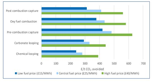
Figure 3.6 Influence of biomass price on cost of carbon avoided on combustion only basis
