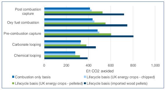
Figure 3.5 Cost of carbon avoided on combustion only and lifecycle basis
