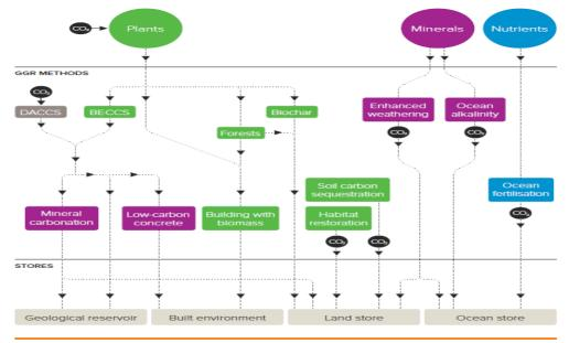
Figure 1.1 Nature-based and technological options for CO<sub>2</sub> removal
