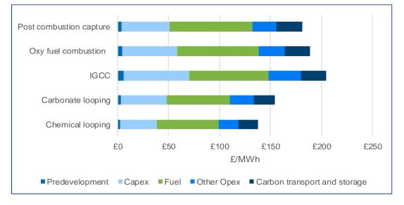
Figure 3.2 Breakdown of LCOE costs for central biomass fuel price (NOAK)
