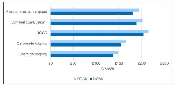
Figure 3.4 Comparison of LCOEs for FOAK and NOAK plant for central biomass price
