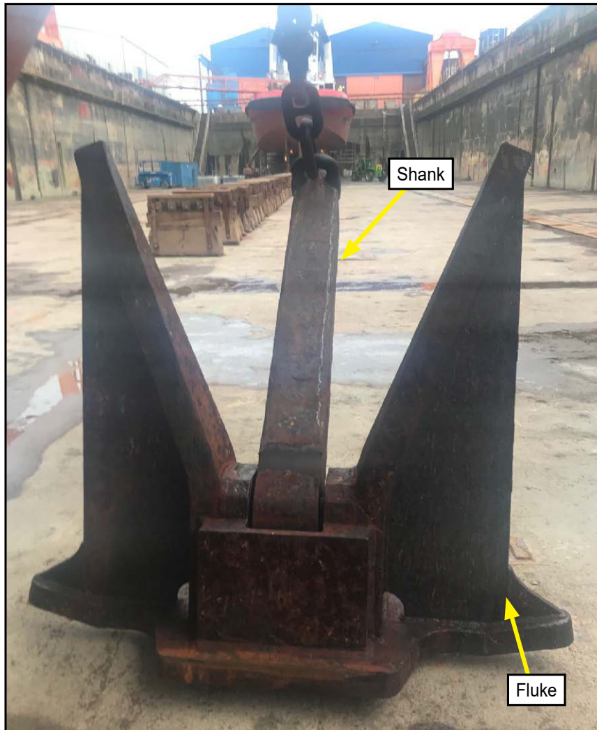
Figure 8: Thea II 's D'Hone, high holding power anchor
