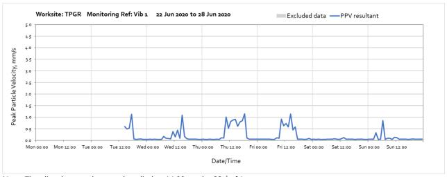
Note: The vibration monitor was installed at 14:00 on the 23<sup>rd</sup> of June.
