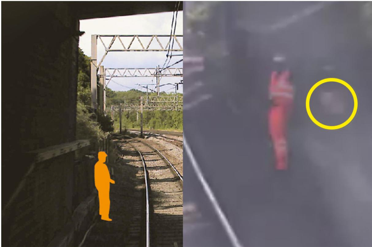
**Images from the front (left) and rear (right) facing closed circuit television system of a northbound train taken at 16:28 hrs, showing the position of the track worker within an area of limited clearance, which is denoted by the sign in the yellow circle (images courtesy of Avanti West Coast).**
