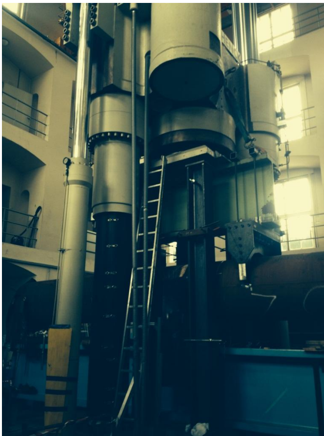
Figure 3 One of the proposed 20MN test rigs for GOAL Grout tests.
