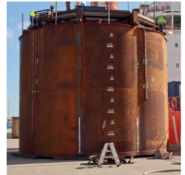
The scaled down Mono Bucket - 8m in diameter with a 6M skirt
