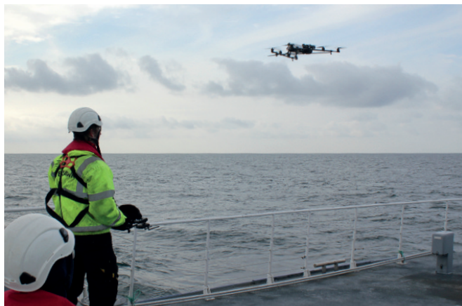
The remotely operated aerial vehicle (ROAV) takes off for the meteorological mast inspection.
