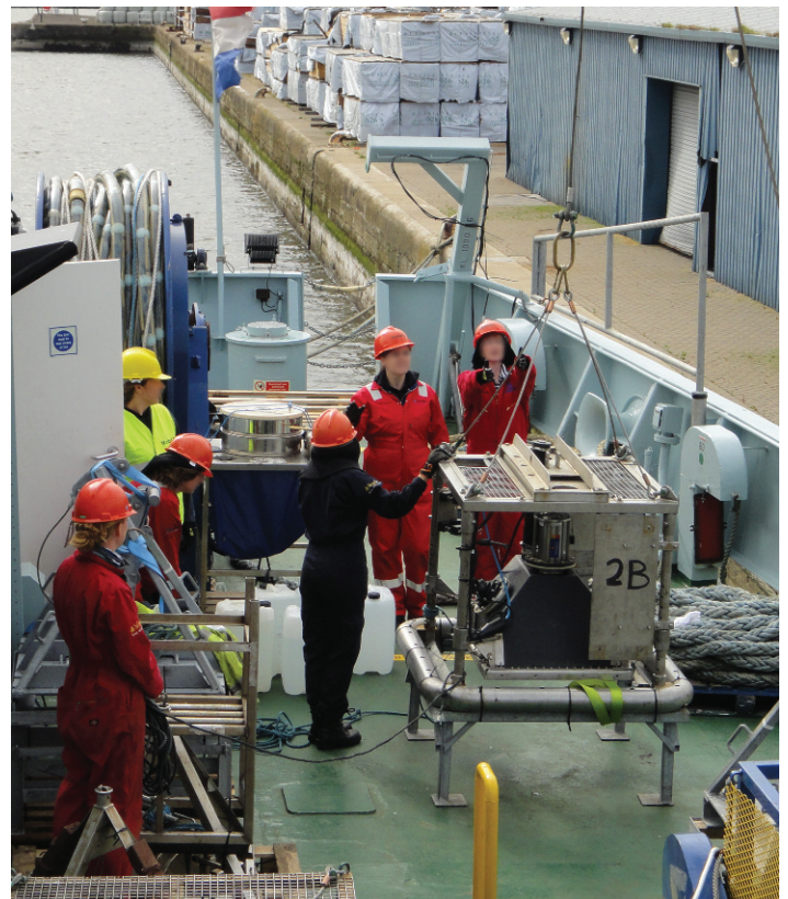
Above: Practice run-through of the use of tag lines during benthic operations identified that it is a more effective methods at times, though use of hands-only is actually preferred in some circumstances.
