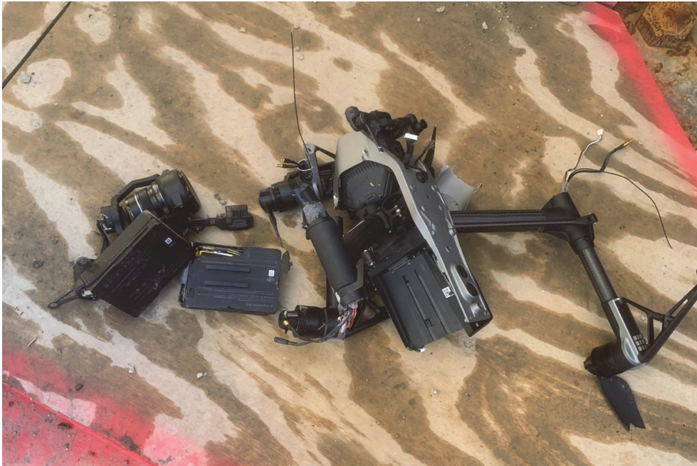
Figure 2 Damage to the drone
